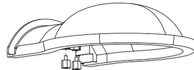
2. Attach TVD-LWB-S to TVD-LWB-2 using the two screws provided (A).
